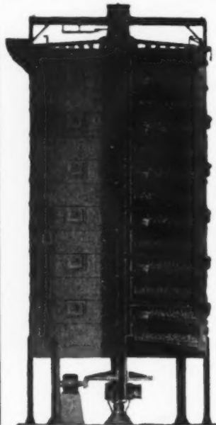
SIZES 8' 6" TO 22' 3" DIAMETER NUMBER OF HEARTHS, 1-16
